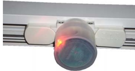
Magnetic field sensor in rail system
